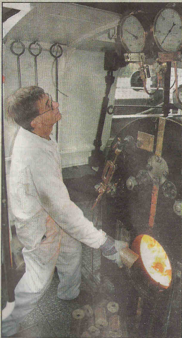
WOOD POWER: One of the new wooden logs is about to be placed into Gondola's boiler
